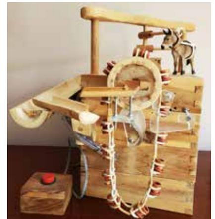
Two of Jan's models: a donkey-powered water-lifting device to irrigate fields, part of a display of working models which included Archimedean screws at the Annual Symposium (*top*), and a trip hammer, modelled after the one in Abinger Hammer and housed in Shere Museum (*bottom*)
