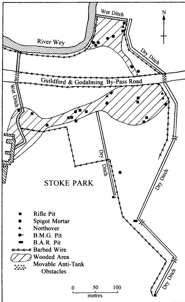
Fig 18.5 Plan of Second World War defences in Stoke Park, Guildford, on either side of the Guildford and Godalming by-pass road, which was opened in 1934. There are 22 rifle pits, four spigot mortars, four Northover projectors, two Bren machine gun pits, one Boys anti-tank rifle pit, about 2km of barbed wire fencing, nearly 1km of dry ditch and about 300m of wet ditch.
