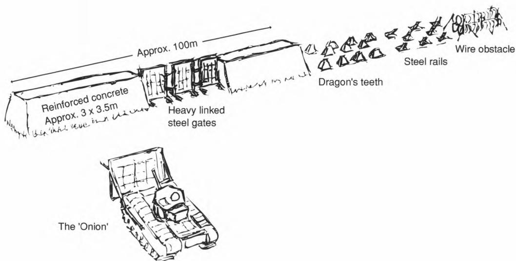
Fig 18.7 Reconstruction sketch of the Atlantic Wall and associated defences at Hankley Common, together with a Churchill tank and its steel frame, 'The Onion'. This sketch is based on one prepared by the driver of the tank (Wood 1988).
