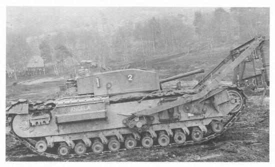
Fig 18.8 Churchill tank equipped with a steel frame capable of placing demolition charges at heights of up to about 4m. Courtesy of the Tank Museum, Bovington, Dorset
