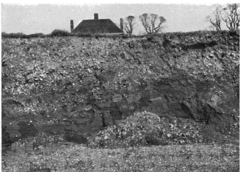
2. Terrace B : Stoneyfield pit, showing stratified gravel and sand overlain by solifluxion gravel. Depth, about 7 feet.
